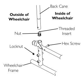
FIGURE 6.1 Installing Back Canes (Lightweight Wheelchair Only)
